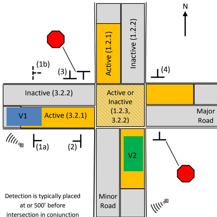
Detection is typically placed at or 500' before intersection in conjunction with static STOP AHEAD warning signs and based on MUTCD Table 2C-4. Guidelines for Advance Placement of Warning Signs
